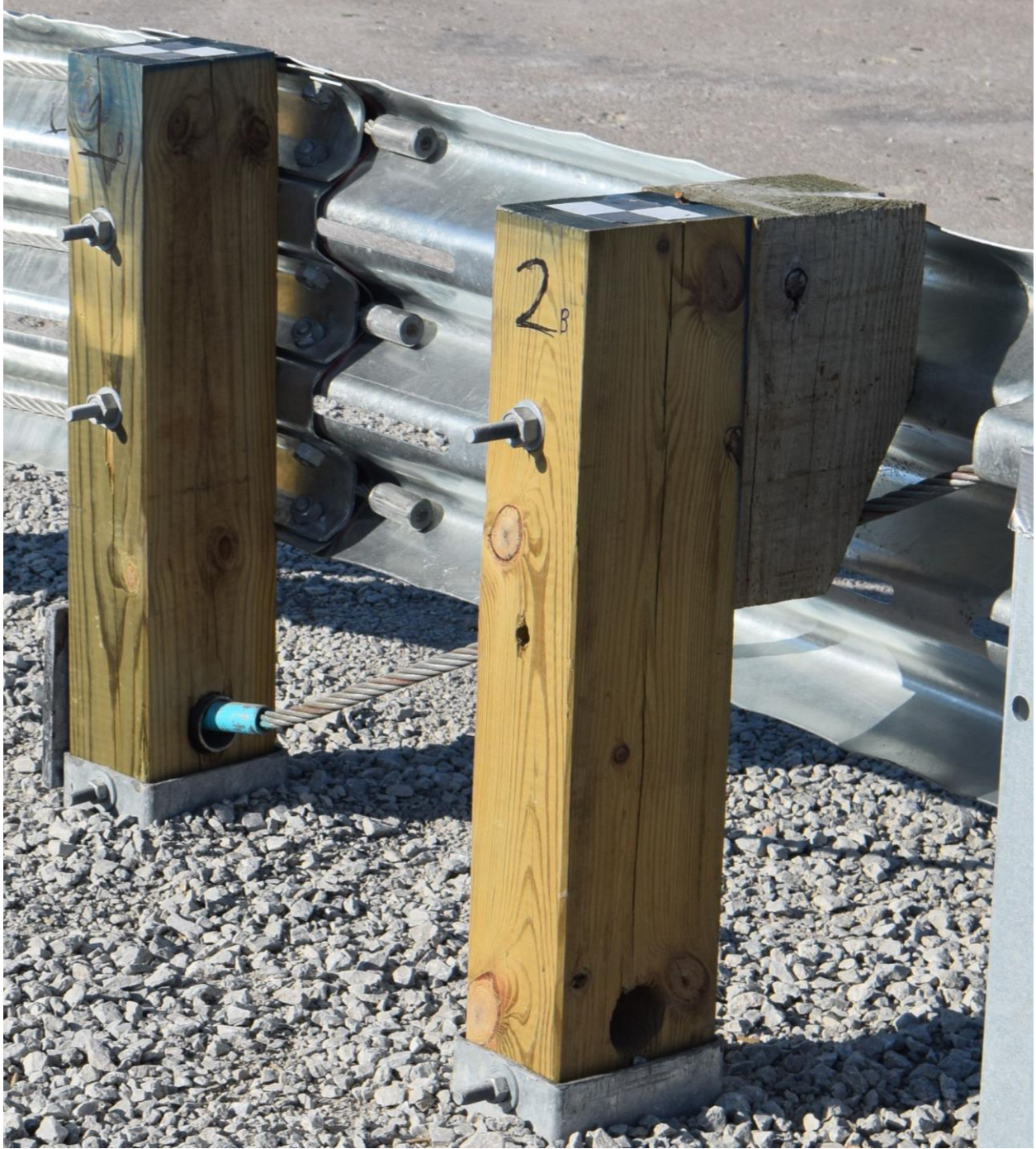
Figure 7. Posts 1 and 2 Installed in System
